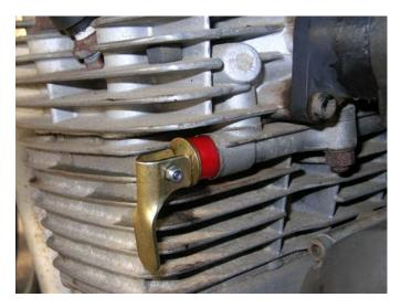
Flip down the trunion (locking) lever to expand the rubber seals and lock the tool into the cylinder. If the tool is not REALLY tight in the YICS passage, remove the tool and tighten the adjusting nut at the end of the tool slightly, put the tool back in and try again. The tool, when locked, should not be movable within nor removable from the passage.
